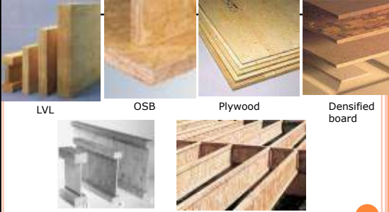
Prefabricated I-joists with laminated veneer lumber flanges and structural panel webs. (A) a hardboard web (B) oriented strandboard and (C) plywood webs.
